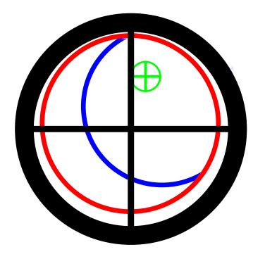
Collimator Secondary Primary Reflected collimator
